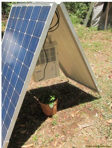
**Making a couple of litres of water from the air** even on the driest of days is easily done with as little as one A-Frame panel set-up, a battery, a small inverter and a compressor dehydrator.
