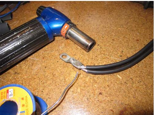
**All plugs and lugs are not just round crimped** (like with most suppliers) but for the longest and most reliable life possible, are flat crimped to increase surface area and then soldered to guarantee optimal contact.
