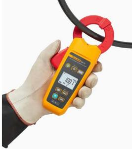
**If we occasionally need to check the battery voltage** or the charging current, we simply use a portable clamp-meter, which is supplied with each kit for free. Charging current is measured by simply putting the clamp around a positive or negative wire to the battery. To work out the power, the current is then multiplied with the battery volts.
