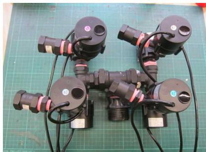
**To avoid any solar energy waste,** multiple water proof, high quality, food grade brushless micro pumps are assembled in series or parallel to meet the exact flow and pressure needs of a specific application.
