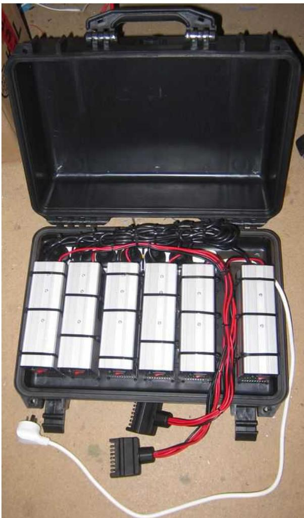
**We supply 1 x 12V or 2 x 12V 60A chargers** built into a solid carry case. Depending on how many chargers are switched on at one time,... 20, 40 or 60A continuous currents can be achieved.
